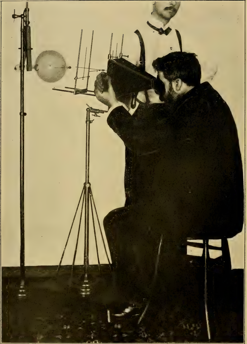
PLATE 64.—Author's One-Minute Localizer locating a bullet in the forearm with a single posturing of patient. Level the markers and tube as taught in the text, press the part on the front marker and screen, shift arm till bullet engages in angle of markers, then—(See next plate for second step).
